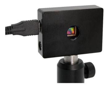
Visualize the beam with real-time ellipse calculations and view cross sections with curve fitting. Key beam width parameters of interest, such as Full Width Half-Maximum (FWHM) and  $1/e^2$  are displayed on the easy-to-use Windows software interface. Track beam centroid stability over time with the beam wander visualization tool featuring customizable test durations and sample rates. Export your results to various image formats or as a PDF report.
